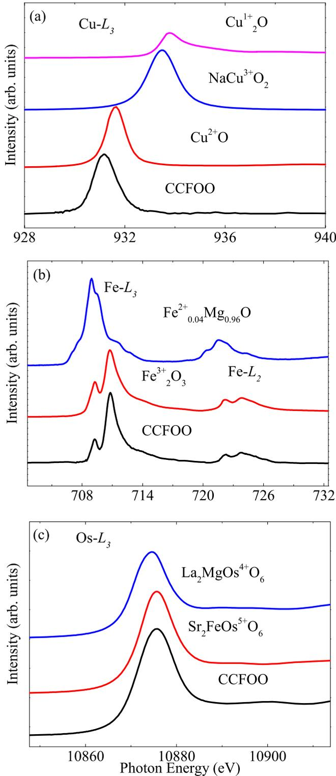
FIG. 2. (a) XAS of Cu- $L_{2,3}$  edges, (b) Fe- $L_{2,3}$  edges, and (c) Os- $L_3$  edges. The XAS of related references are also shown for comparison.
